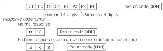
When more than one code is being sent, send each command only after the OK response code for the previous command from the unit is verified.
